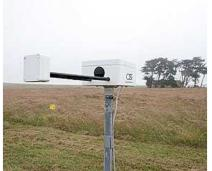
Optical rain gauge (source: The Atmospheric Radiation Measurement (ARM) Program)
