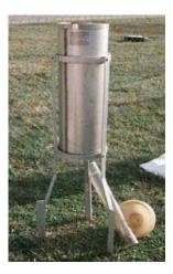
Figure 1.1: The National Weather Service Standard Rain Gauge, SRG (source: <u>http://www.srh.noaa.gov/tlh/cpm/srg\_page.html</u>
