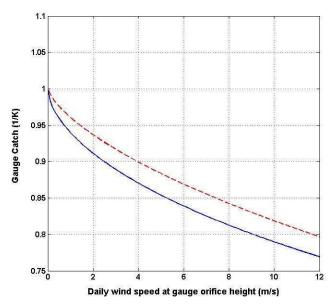
Gauge catch due to wind effect for gauges without wind-shield (solid line) and with wind-shield (dotted line).
