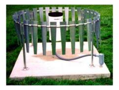
An example of wind-shield installed to reduce wind effect on rain gauge measurements (source: NovaLynx Corporation)
