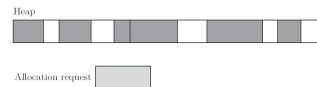
Figure 3.3: External fragmentation. The shaded blocks are in use; the clear blocks are free. While there is more than enough total free space remaining to satisfy an allocation request of the illustrated size, no single remaining block is large enough.
