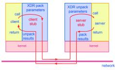
Each RPC invocation by a client process calls a *client stub*, which builds a message and sends it to a *server stub*
