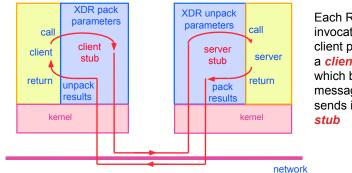
Each RPC invocation by a client process calls a *client stub*, which builds a message and sends it to a *server stub*
