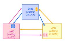
A cycle of LPs forms where each is waiting on the next LP in the cycle. No LP can advance; the simulation is deadlocked.
