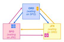
A cycle of LPs forms where each is waiting on the next LP in the cycle. No LP can advance; the simulation is deadlocked.
