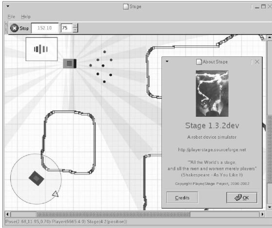
**Figure 2:** Stage screenshot showing two robots (solid rectangles) with visualization of the top robot’s laser range scanner, sonar and color blob-finder data. Stage’s modular architecture allows multiple GUIs; this is GNOME2.
