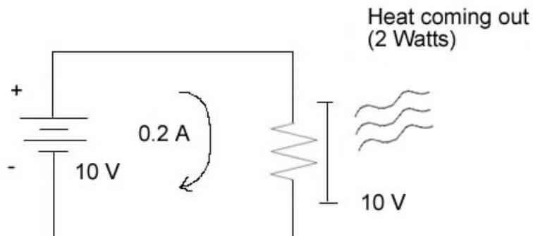
Resistors are rated for the maximum wattage they can carry without harm (usually  $1/8\text{ W}$ ).
