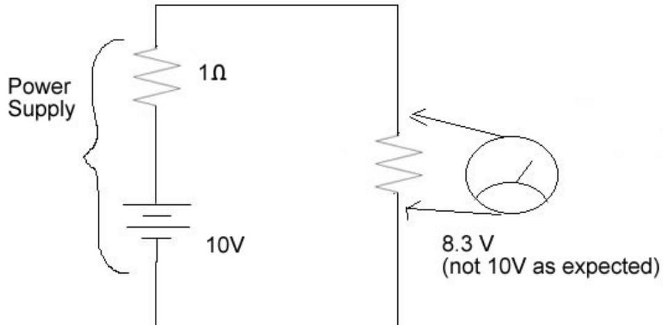
The internal resistance of a lab-type power supply is about  $0.1\ \Omega$ . That of a 9-volt battery can be as high as  $100\ \Omega$ .
