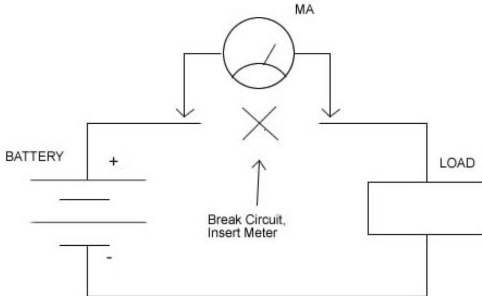
**SAFETY:** Remember, **a current meter conducts electricity!** Don't connect it anywhere you wouldn't connect a piece of wire.
