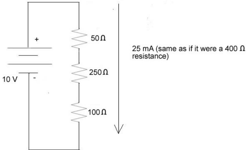
Since each resistor conducts the total current, it follows that each resistor does not experience the total voltage. (If it did, Ohm's law would be violated.) Instead, the **voltage is divided among the resistors**.
