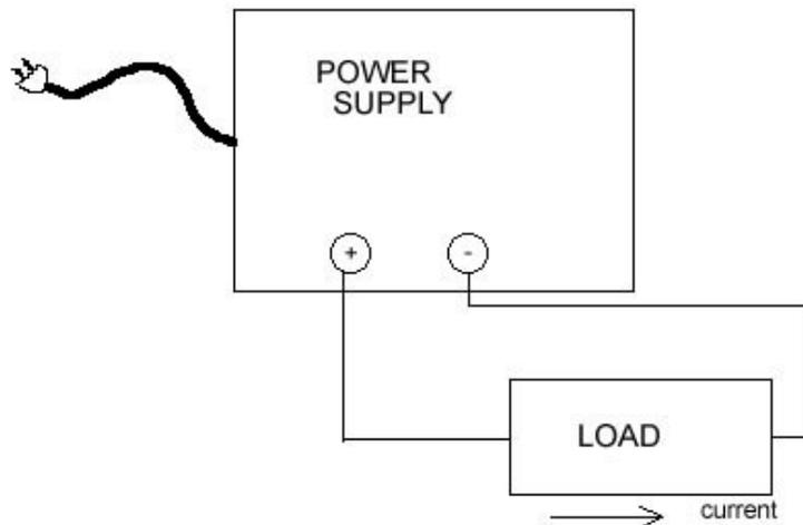
**SAFETY: Never allow electricity to flow from + to - without going through a suitable load!** If you do, you’ll have a *short circuit* and things may burn up.
