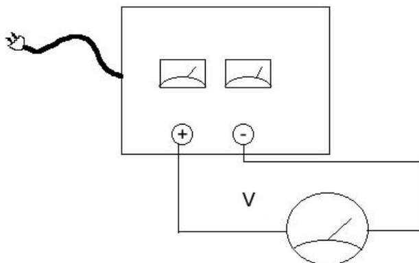
METER MUST be set to measure voltage BEFORE you connect it to the circuit.
