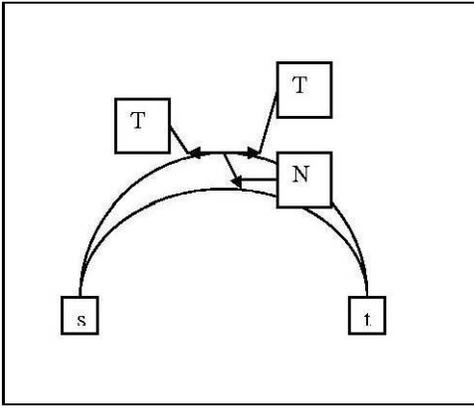
**Fig. 1.** A 2D flow network with a source  $s$ , a sink  $t$  and typical tangential ( $T$ ) and normal ( $N$ ) edges.
