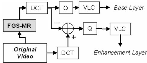
**Figure 1: A basic MPEG-4 FGS scalable video encoding pipeline, with the proposed FGS-MR step added (in the shaded box).**
