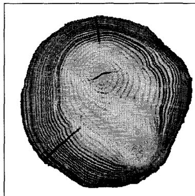
**Figure 11.** An image of Oak may cause the segmentation algorithm to fail to retain the knot region.
