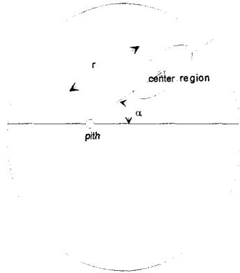
**Figure 8.** The two geometric values used to group the defect-like regions.
