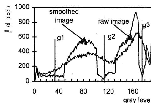
Figure 3. Histogram of the image and threshold selection.
