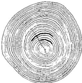
Fig. 17. Results of the grayscale histogram-based crack extraction procedure.
