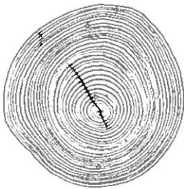
Fig. 16. Identification and localization of the actual crack defect.
