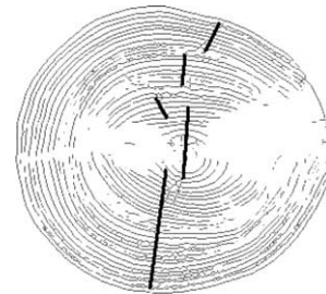
Fig. 18. Results of the proposed crack detection procedure on the second CT image.
