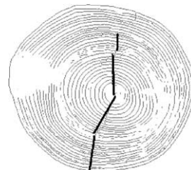
Fig. 19. Results of the proposed crack detection procedure on the third CT image.
