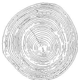
Fig. 8. Result of the thinning algorithm.
