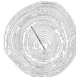
Fig. 15. The result of the RANSAC-based line fitting to the detected fork pixels.
