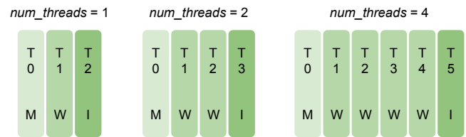
Figure 4: The actual number of threads created by the benchmark bodytrack in PARSEC is different from the number of threads specified by the input parameter num_threads . M: main thread, W: worker thread, I: I/O thread.
