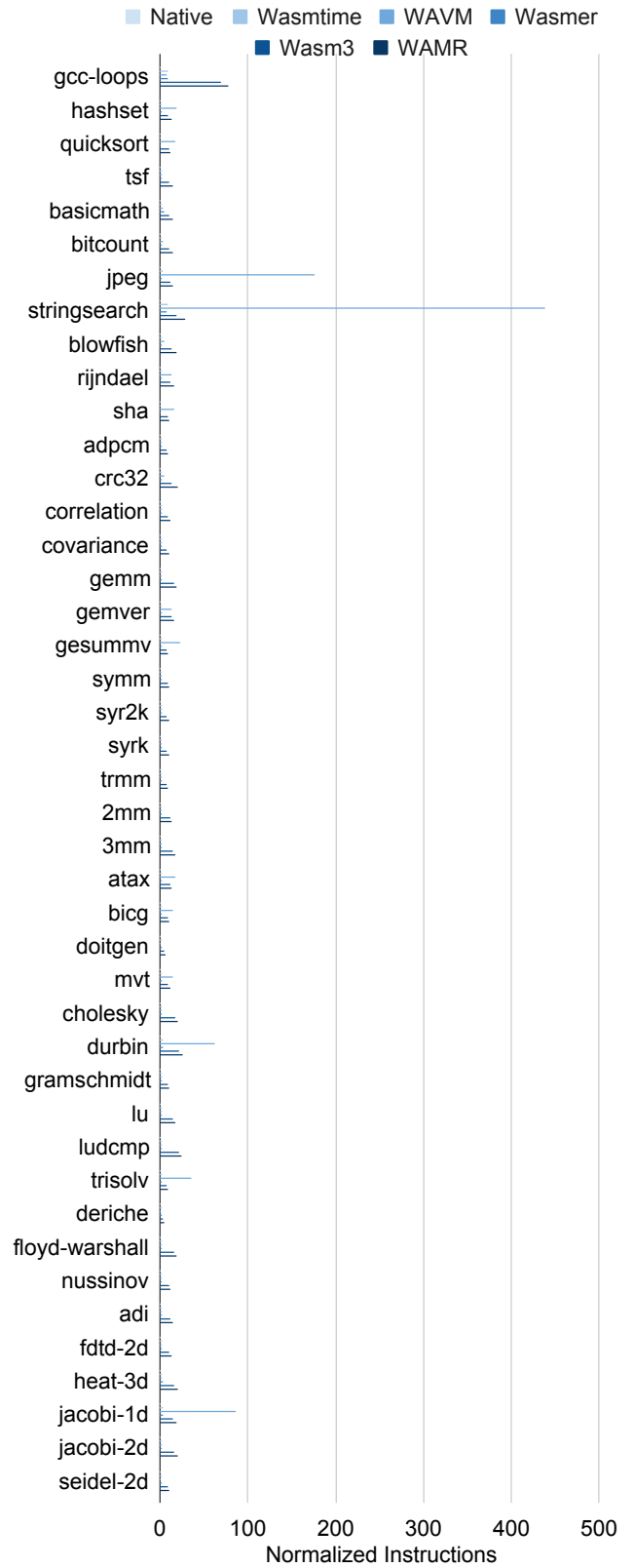
Figure 14: Normalized numbers of dynamic instructions of WebAssembly runtimes for benchmarks in JetStream2, MiBench, and PolyBench. The baseline is native execution.
